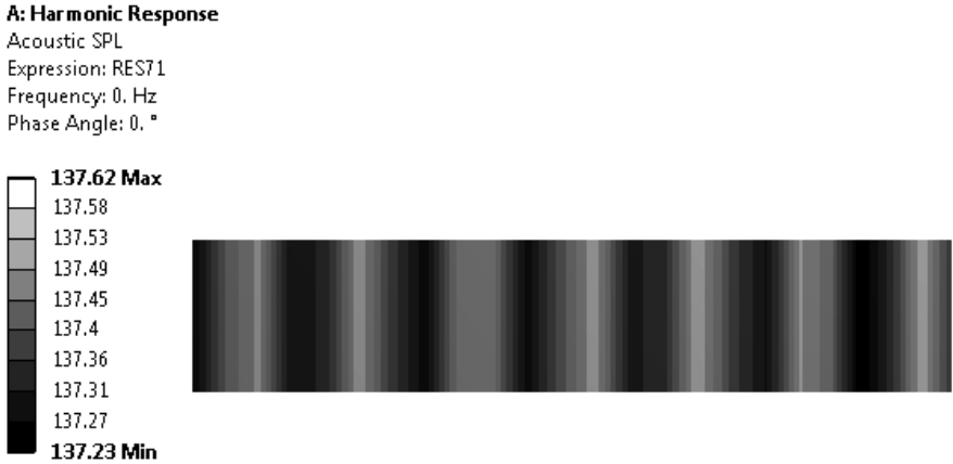
FIGURE 3.35 Case (A): Sound pressure level at 600 Hz using a FLUID30 mesh shown in Figure 3.34.
